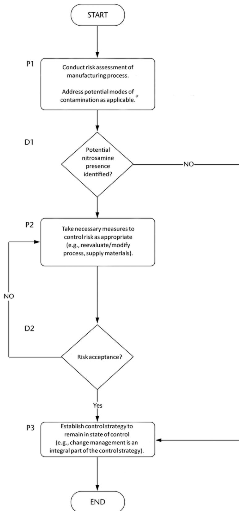
Figure 3. High level process for development of a nitrosamine impurity control strategy. (ªRefer to [Table 2](#); P1, P2, P3 = Process 1, 2, 3; D1, D2 = Decision 1, 2)
